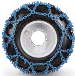
Front side without tensioning chain
